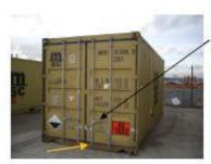
Container seals have to be fitted at the right container door - the inner locking bar /handle- only. Or as shown right to the right inner bottom locking cam
